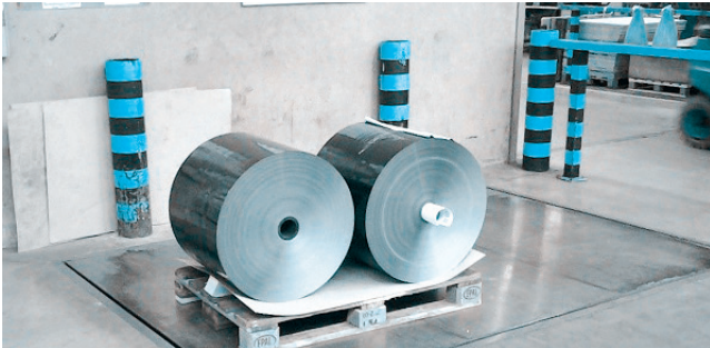
Load weight is checked when the load is picked up
